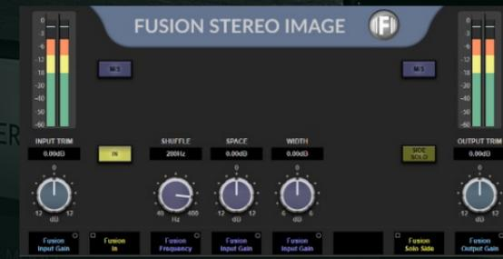
**Stereo Image** enhancer provides a Mid-Side circuit that manipulates the Side signal, allowing for widening and spatial manipulation of the stereo field. The 'Space' circuit is a frequency-dependent width control based on the concept of Stereo Shuffling, allowing injection of interesting depth effects into the mix. Stereo Image exposes a 'Shuffle' control for changing the frequency cut-off in the Space circuit, allowing you to add weight and presence or carve space in the stereo field.
