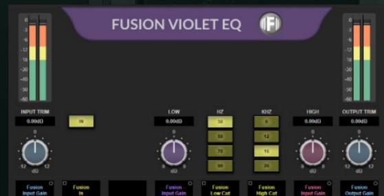
**Violet EQ** is an all-new minimum phase-shift, two-band shelving EQ. It draws on the SSL legacy of carefully selected frequencies and response curves to create a musical and intuitive EQ designed to quickly dial in low-end weight and high-end sheen. High and Low frequency circuits each offer four switched high-frequency points and +/-9dB attenuation.
