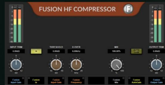
**High Frequency Compressor** recreates the distinctive high frequency smoothing circuit from SSL Fusion. A compressor that effects high frequencies only, optimised for smooth and transparent harshness reduction and a tape-like high-frequency roll off – great for taming brittle high frequency fizz.
