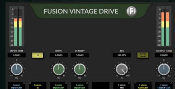
**Vintage Drive** is a unique non-linear harmonic enhancement circuit that brings cohesion and strength to your mix. Drive and Density controls interact to produce harmonic saturation and soft compression derived from overloading an analogue circuit. It can be used lightly for subtle thickening saturation or driven hard for more extreme distortion.
